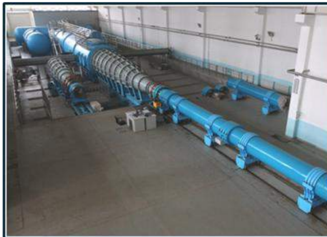
Figure 6 – CAS IOM JF-12 Shock Tunnel, Duplicating Hypersonic Flight Conditions at Mach 5 – Mach 9 283
